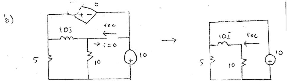
$$\begin{aligned} \therefore V_{oc} &= \frac{10j}{10 + 10j} \cdot 10 \\ &= \frac{10j}{1+j} \end{aligned}$$
