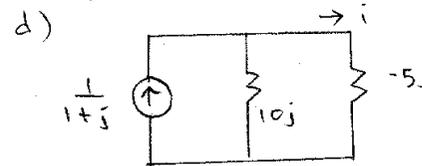
$$\begin{aligned} \therefore i &= \frac{1}{1+j} \cdot \frac{10j}{10j - 5j} = \frac{2}{1+j} \\ &= \frac{2}{\sqrt{2} \angle 45} = \sqrt{2} \angle -45 \end{aligned}$$
