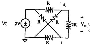
$$\text{Q.a: } \frac{V_i - V_a}{R} = \frac{V_a - V_b}{2R} + \frac{V_b}{R}$$
