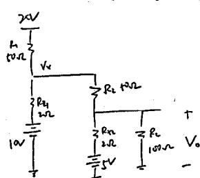
$$\frac{20 - V_x}{50} = \frac{V_x - 10}{2} + \frac{V_x - V_0}{50} \Rightarrow 20 - V_x = 25V_x - 250 + V_x - V_0 \\ \Rightarrow 270 = 27V_x - V_0 \quad \textcircled{1}$$
