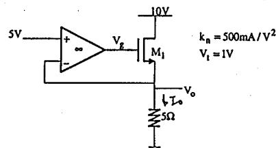
Ideal op-amp  $\Rightarrow V_o = V_- = V_+ = \frac{1}{2}V$ .
