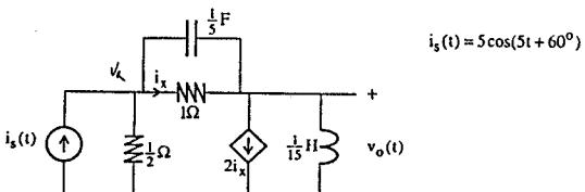
$$\textcircled{1} \quad @ V_a = i_s = \frac{V_a}{\frac{1}{5F}} + \frac{V_a - V_o}{j\frac{1}{F}} + \frac{V_a - V_o}{1} \\ \Rightarrow i_s = 2V_a + j(V_a - V_o) + V_a - V_o$$
