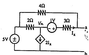
$$V_{oc} = \frac{5 - V_a}{2} = 2I_x + I_x = 3I_x \quad \textcircled{1}$$
