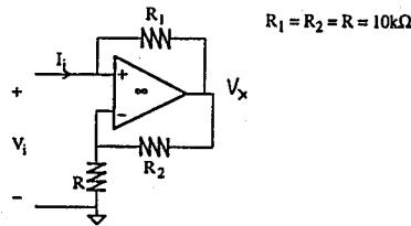
$$V_- = \frac{R}{R+R_2} V_x = V_i$$
