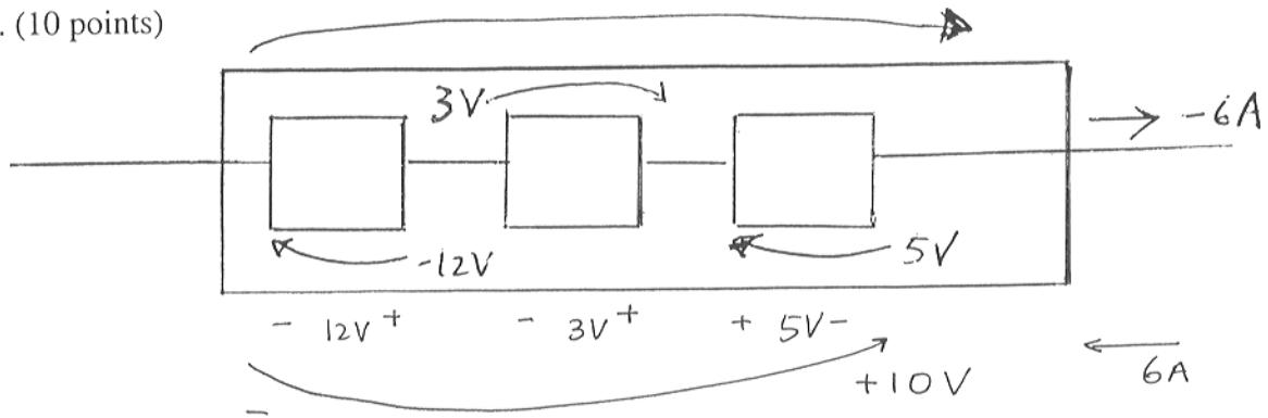
By definition, current flowing into the (+) terminal of an element is (+). The element is passive since current flows in at higher potential and leave at lower potential. Power absorbed =  $10 \times 6 = 60 \text{ W}$
