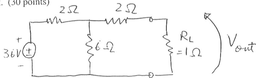
$$(a) V_{oc} = \frac{6}{6+2} \times 36 \text{ V} = 27 \text{ V}$$
