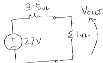
$$V_{out} = \frac{1}{1+3.5} \times 27 = 6 \text{ V}$$
